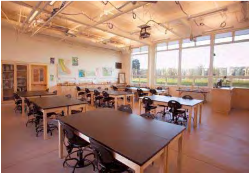
Ceiling fans and operable windows to maximize daylight and natural ventilation
